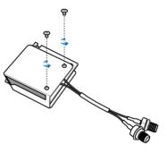
2. Remove the long screw at the front, then remove the metal cover.
